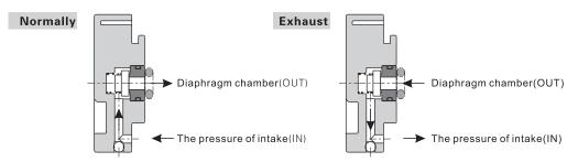
Normally, as the pressure of intake (IN) is higher than the set valve(pressure of outlet), the reverse flow valve closed; if the pressure of intake(IN) is cut off and starts exhaust, reverse flow valve opens. The pressure of diaphragm chamber is exhausted from IN orifice. At this moment, the pressure of diaphragm chamber decreases and the diaphragm is pressed down by the force from adjusting spring to open valve. The pressure from outlet is exhausted from IN port.
